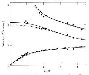
FIG. 2. Measured velocity in unsupported Au films as a function of the product of the thickness (d) and wave vector  $(q_{\parallel})$ . The full and dashed lines are fits based on hexagonal or isotropic symmetry of the Au layer.
